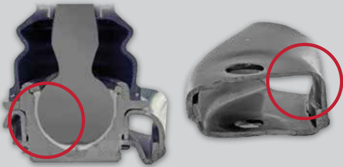
CONTROL ARM BODY Key support areas of control arm body are hollow
