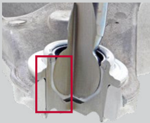
BALL JOINT Sealed plastic bearing design
