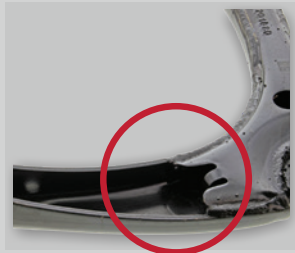
CONTROL ARM BODY Control arm body uses partial clamshell stamped steel design
