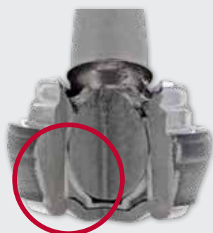
OEM OUTER TIE ROD Non-greaseable plastic bearing
