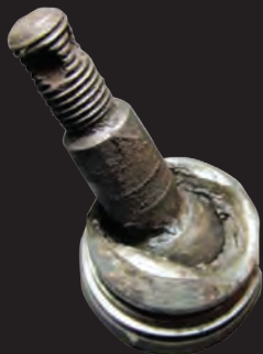
Housing is used as stud contact surface
