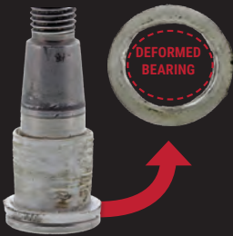
Constant off-centre loading can deform bearing
