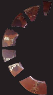
Failed Spring Disc
