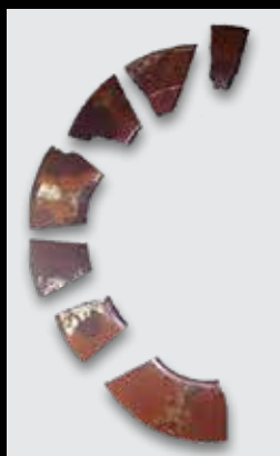
Failed Spring Disc
