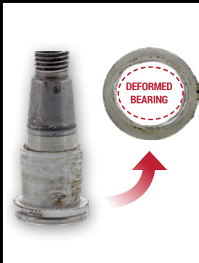
Constant off-centre loading can deform bearing
