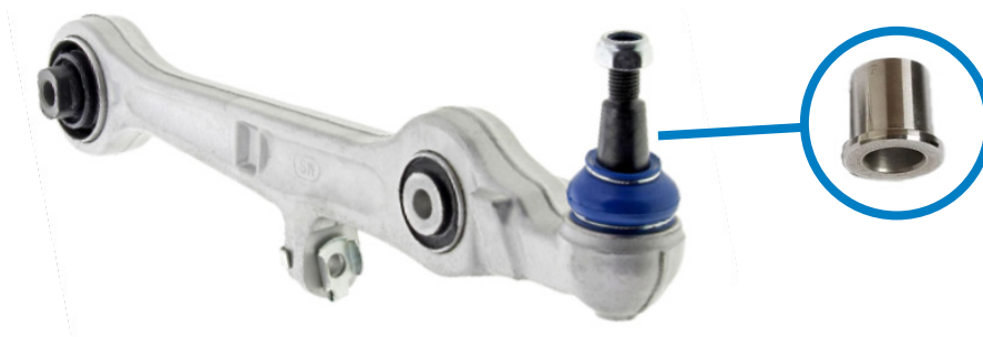
Figure 1. Steering knuckle tapered sleeve (circled) may become seized to the ball joint stud, and when compared to the new replacement part cause a visual difference between the two. Mevotech Supreme control arm assemblies feature an anti-corrosion coated ball stud to reduce potential of seizing.
