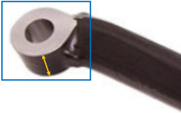
Figure 1. First design “thin” neck front lower forward control arm
