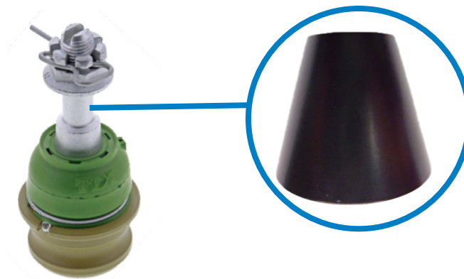
Figure 1. Ball seating cone (circled) may become seized to the ball joint stud, causing it to appear different than the Mevotech part. Mevotech replacement ball joints with the part numbers TXK9513/MK9513/GK9513 feature an anti-corrosion coated ball stud to reduce the potential of seizing.
