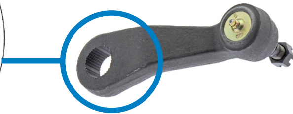
Figure 2. Pitman arm with 4 grooves
