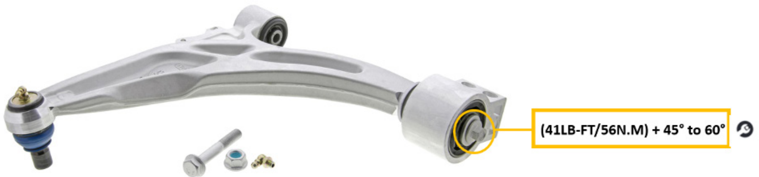
Figure 1. Bushing bracket bolt (circled above) must be correctly torqued after fitting control arm to vehicle
