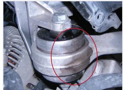
Figure 1: Hydraulic fluid leaking from bushing. One indicator of failed bushing.
