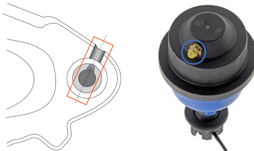
Figure 1. To ensure adequate clearance between components and accessibility for future relubrication service, ball joint must be installed with grease fitting in alignment to channel groove on front lower control arm
