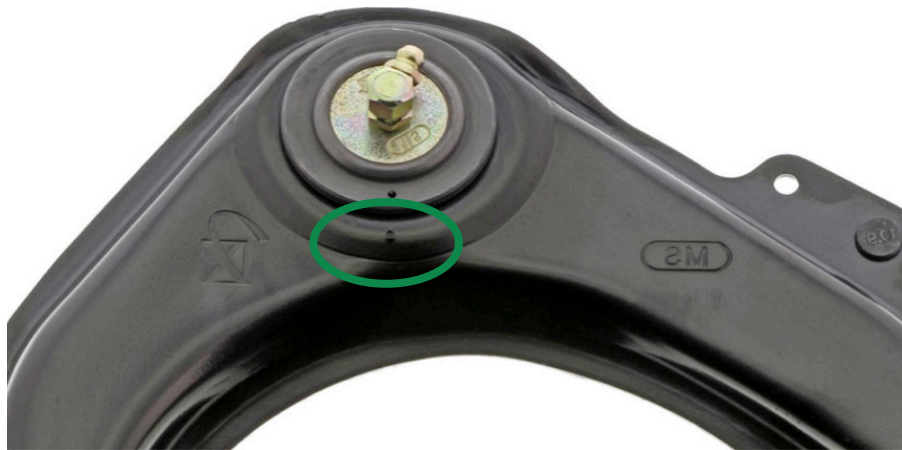
Figure 2. Control arm index mark. In this example, the index mark is a hole.
