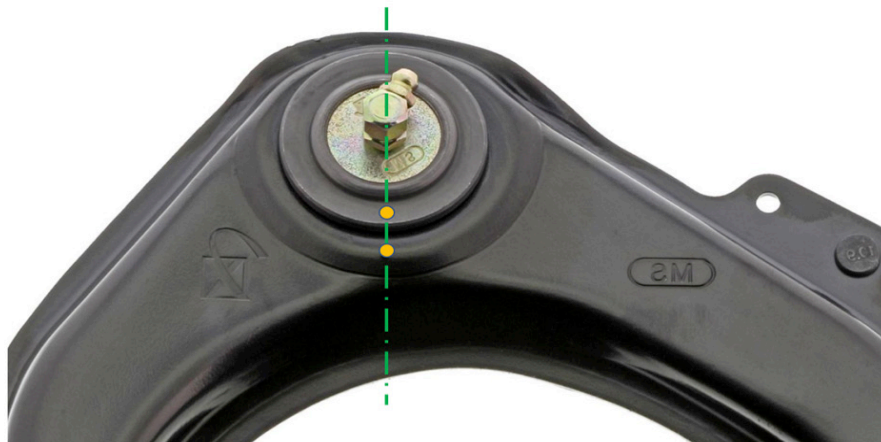
Figure 3. Correct installation orientation is achieved when ball joint index mark aligns with control arm side index mark.
