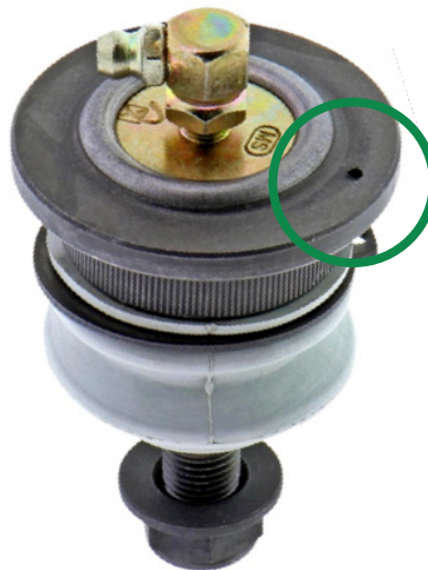
Figure 1. Ball joint index mark. In this example, the index mark is a hole.
