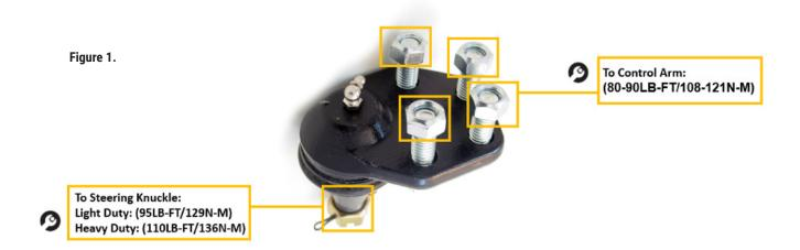
Always ensure to refer to the factory service manual for correct diagnostic procedures, component removal and installation methods and fastening torque values and procedures where applicable. Only use a calibrated torque wrench for final fastening.
