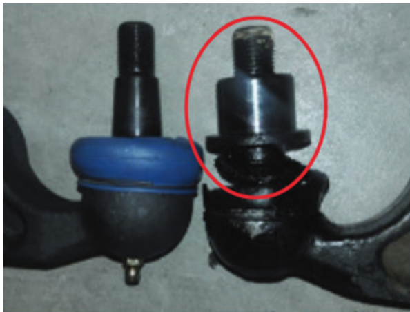
Figure 1. Original control arm with insert seized to stud (circled in red).
