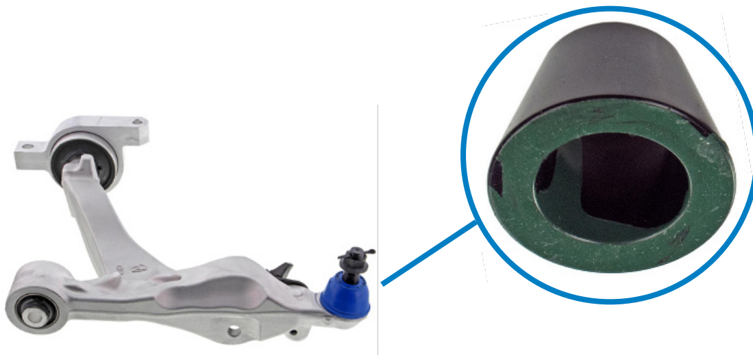
Figure 1. Typical Nissan and Infiniti ball joint seating cone (circled). This cone may become seized to the ball joint stud and cause a visual discrepancy when compared to the new replacement control arm.
