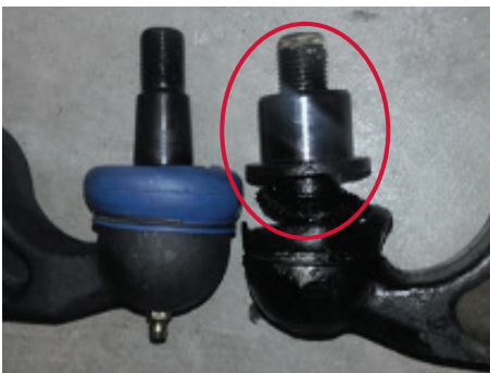
Figure 1: Seized insert (circled) on original control arm stud
