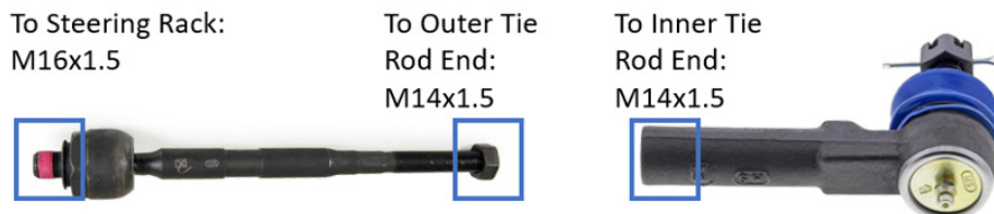
Figure 1. If M14 components are required, use the following Mevotech Supreme replacement inner and outer tie rod ends after confirming vehicle trim and package:
