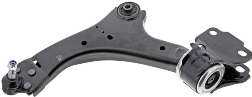
Figure 1. Type 1: Stamped steel construction and riveted ball joint
