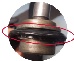
Figure 1: Deformed Control Arm
