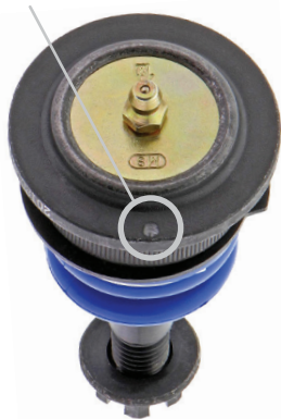
Figure 1 - Drilled Index Mark
