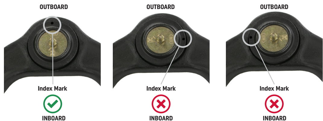
Figure 2 - Correct Installation Orientation
