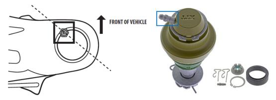
**Figure 1.** To ensure adequate clearance between components for relubrication service, ball joint must be installed with grease fitting positioned approximately 45° towards centerline of vehicle. Grease fitting must also be positioned facing front of vehicle.
