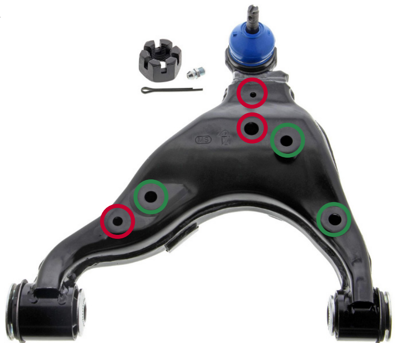
Figure 1. Correct rubber plug installation locations (circled in green). To ensure adequate drainage, do not cover or attempt to install plugs at locations circled in red
