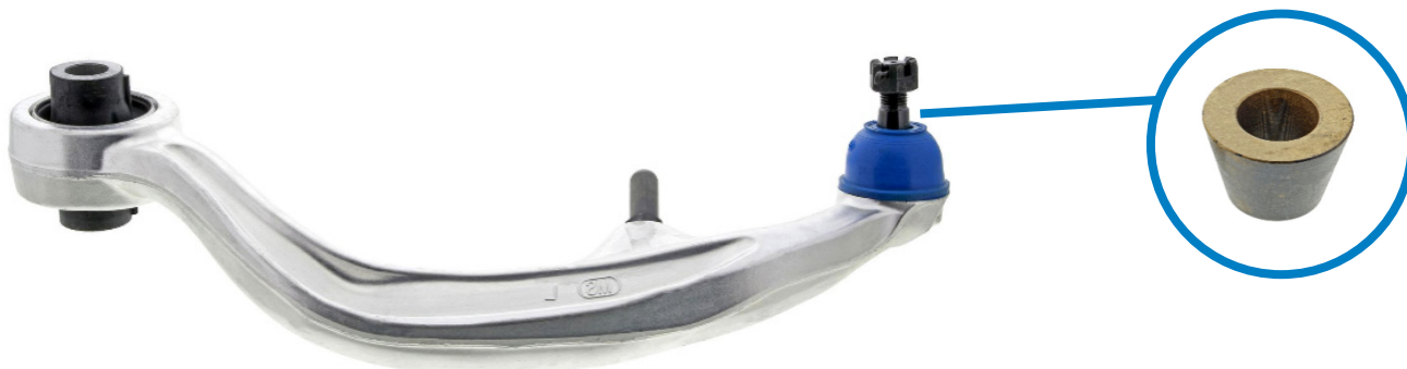
Figure 1. Tapered sleeve (circled) may become seized to the ball joint portion of the old control arm, and when compared to the new replacement part cause a visual difference between the two. Mevotech Supreme front lower rearward control arms CMS30165 and CMS30166 are anti-corrosion coated to reduce potential of seizing.
