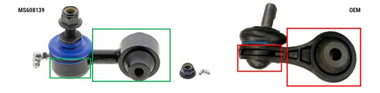
**Figure 1.** Mevotech Supreme MS608139 rear stabilizer bar link with solid steel body, featuring greaseable, self-lubricating sintered bearings, increased ball pin to bearing contact area and included hardware (left) vs OEM plastic body and sealed plastic housing (right)
