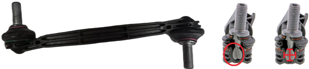
Figure 1. Mevotech Supreme MS258151 with solid steel design, featuring greaseable, self-lubricating upper and lower sintered metal bearings, increased ball pin to bearing contact area and included hardware (top) vs OEM plastic body, sealed plastic housing and reduced ball pin contact area (bottom)
