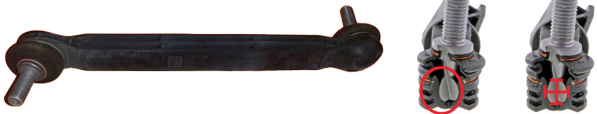
Figure 1. Mevotech Supreme MS258135 with solid steel design, featuring greaseable, self-lubricating upper and lower sintered metal bearings, increased ball pin to bearing contact area and included hardware (top) vs OEM plastic body, sealed plastic housing and reduced ball pin contact area (bottom)
