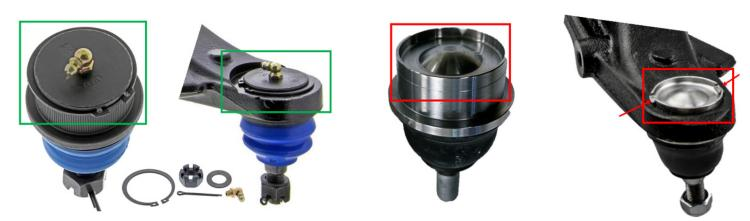
Figure 1. Mevotech Supreme front lower ball joint MK80629 can be secured to the control arm easily via the included circlip (left) vs OEM stake/crimp method (right)
