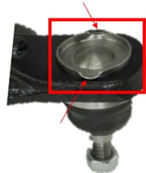
**Figure 1.** Mevotech Supreme front lower ball joint MK80629 can be secured to the control arm easily via the included circlip (left) vs OEM stake/crimp method (right)
