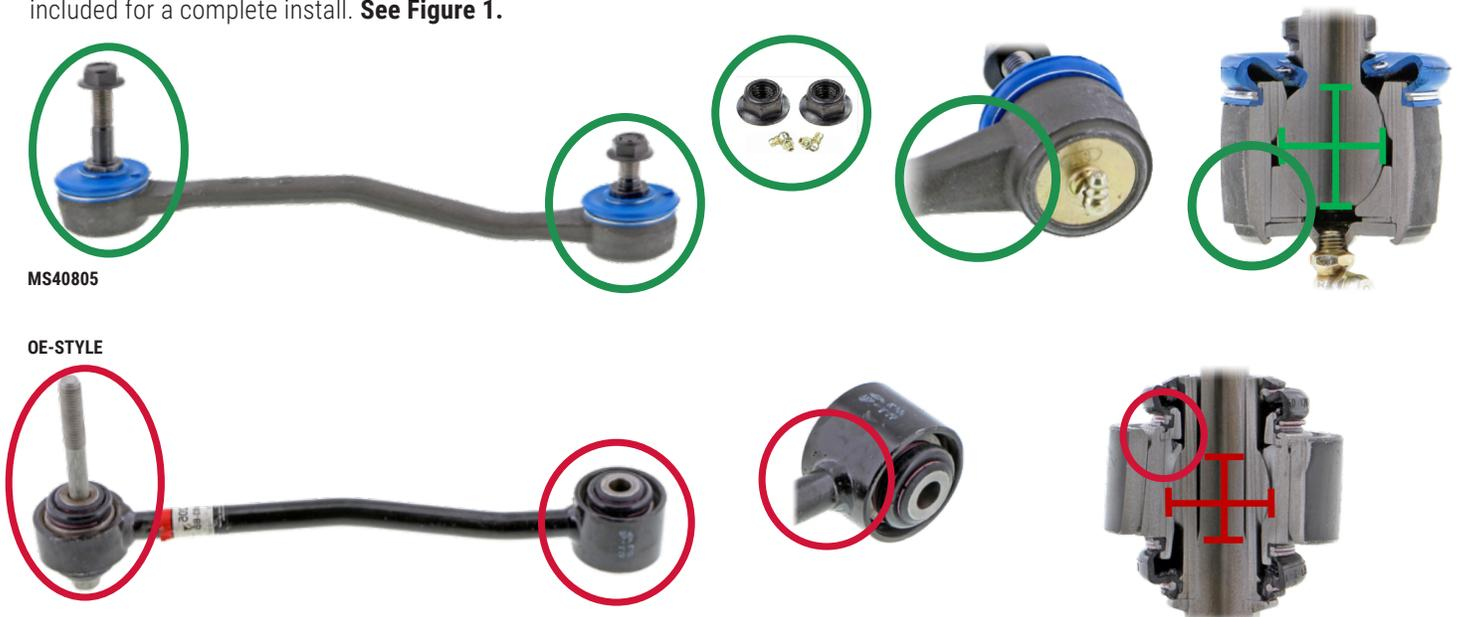
**Figure 1.** Mevotech Supreme front stabilizer link MS40805 with solid steel 1-piece forging and integrated ball joints, featuring greaseable, self-lubricating lower sintered metal bearing, increased ball pin to bearing contact area and included hardware (top) vs OEM with bushings design, sealed plastic bearing, welded connection and reduced ball pin contact area (bottom)
