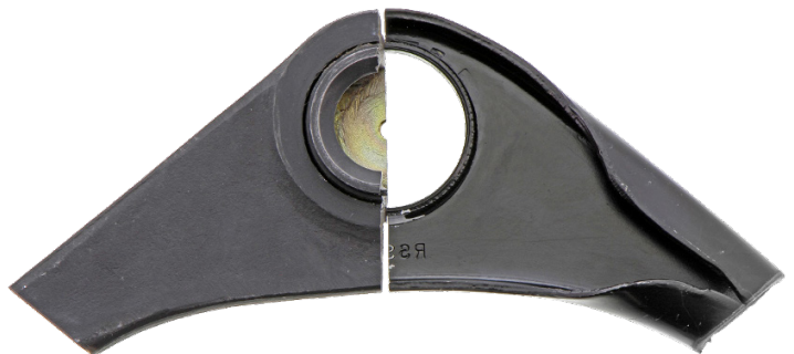
Figure 2 : Mevotech reinforced solid forged control arm neck (left) vs OE stamped steel (right)
