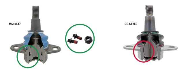
Figure 1. Mevotech Supreme MS10547 with self-lubricating sintered upper and lower metal bearings and included hardware (left) vs 0E-style ball joint with plastic bearing and uncoated components (right)
