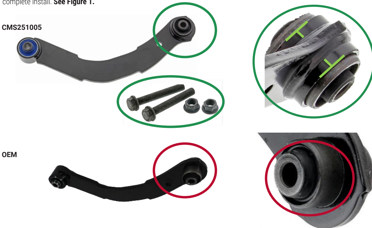
Figure 1. Mevotech Supreme control arm CMS251005 with improved stamping profile and included hardware (top) vs OEM design (bottom)
