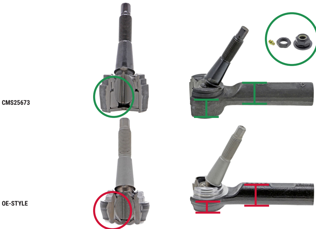
Figure 1. Mevotech Supreme outer tie rod end MS25673 with improved forging profile featuring greaseable self-lubricating sintered upper and lower metal bearings and included hardware (top) vs OEM design (bottom)
