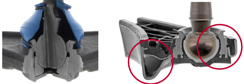
Figure 2 : Mevotech upper and lower sintered metal bearings (left) vs OE plastic “liner” style bearing with voids in key support areas (right)
