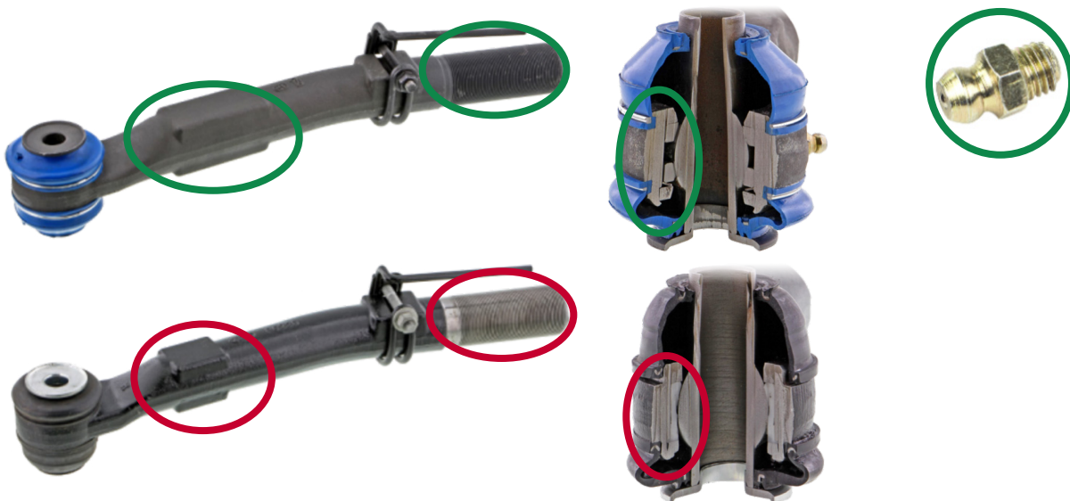
Figure 1. Mevotech Supreme front right outer tie rod end MS40672 with improved forging profile, featuring greaseable, self-lubricating upper and lower sintered metal bearings, anti-corrosion coating and included hardware (top) vs OEM with sealed plastic bearing, reduced forging profile and uncoated finish on threaded end (bottom)
