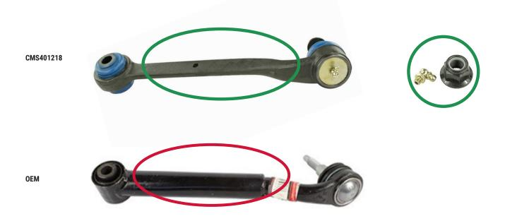
**Figure 1.** Mevotech Supreme control arm CMS401218 with improved solid forged steel profile featuring greaseable self-lubricating sintered metal bearings and included hardware (top) vs OEM hollow stamped steel tube and non-serviceable ball joint (bottom)
