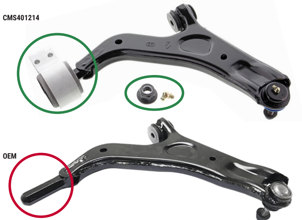
Figure 1. Mevotech Supreme front lower control arm assembly CMS401214 with pre-fitted bushing and hardware (top) vs OE-style bare control arm (bottom)
