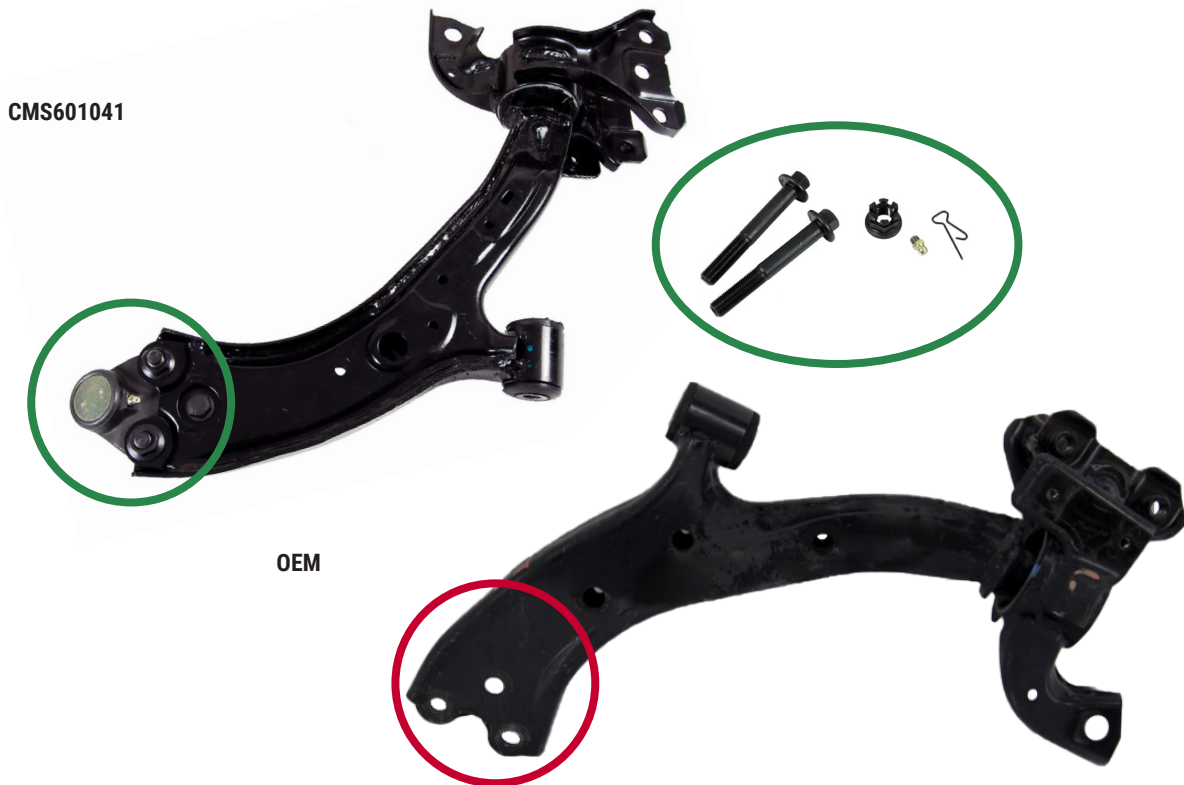
Figure 1. Mevotech Supreme front lower forward control arm CMS601041 pre-fitted ball joint and hardware (top) vs. OEM bare control arm (bottom)
