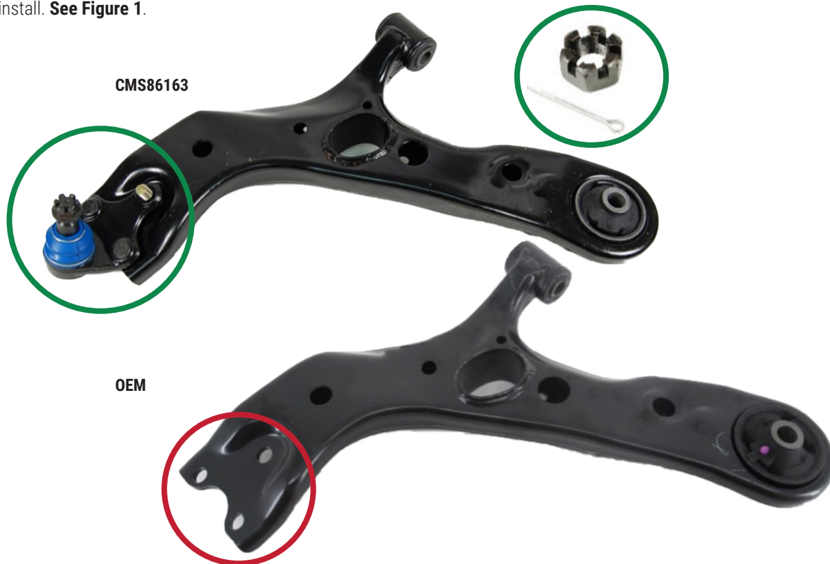
Figure 1. Mevotech Supreme front lower control arm assembly CMS86163 with pre-fitted ball joint and hardware (top) vs OEM control arm (bottom)
