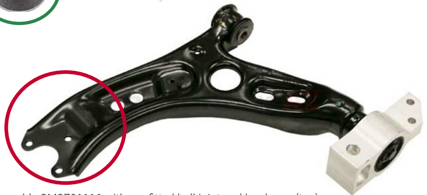
Figure 1. Mevotech Supreme front lower control arm assembly CMS701116 with pre-fitted ball joint and hardware (top) vs OEM control arm (bottom)
