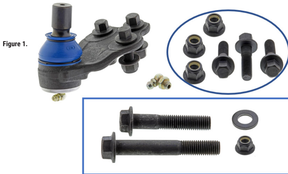
Figure 1. Mevotech Supreme front lower ball joint MS25548 with full hardware kit, including pinch bolts, washer, and nut to steering knuckle (highlighted in square callout box) and bolts and nuts to control arm (circled)
