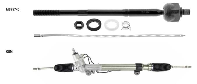
Figure 1. Mevotech Supreme front inner tie rod end MS25740 with included hardware (top) vs OEM steering rack (bottom)
